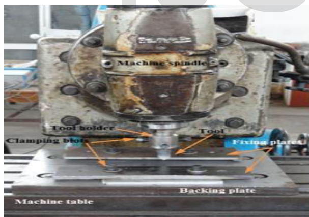
Fig. 3. FSW setup on milling machine
